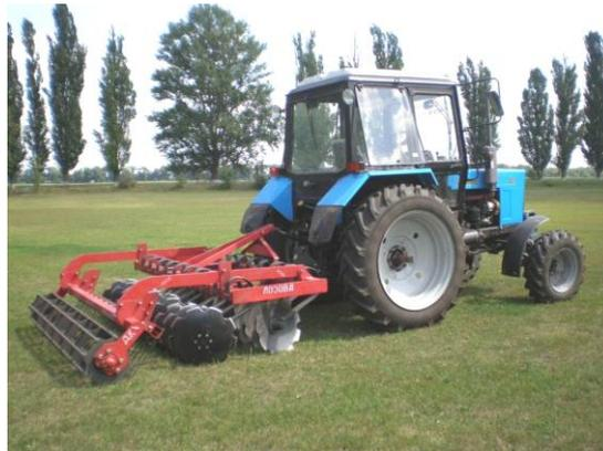
**Fig. 3.3 - General view of a disk header with spring shanks**
