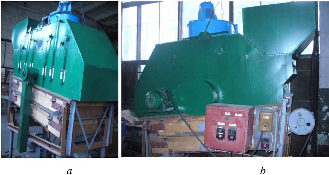
**Fig. 4.3. Design of the modernized aspiration chamber of the flat-radiator separator and its general appearance (a, b).**
