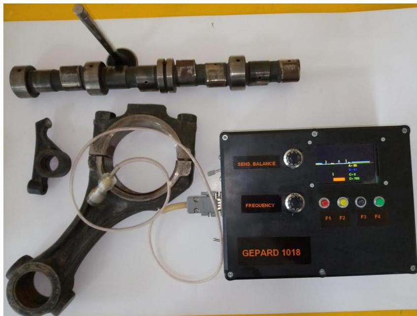
**Fig. 11.1. Portable eddy-current defectoscope**
