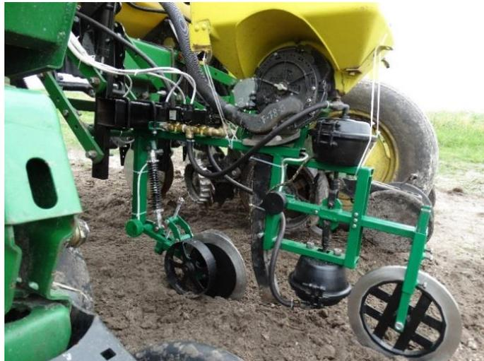
**Fig. 2.6 - A two-phase coultter system on John Deere 7000 planter**
