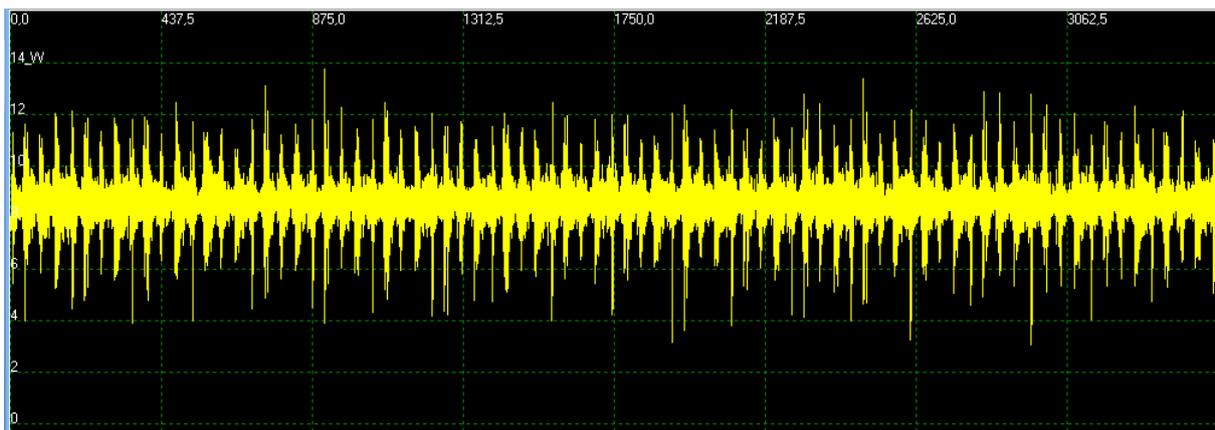
**Fig. 5.4. Work of the second cylinder nozzle**
